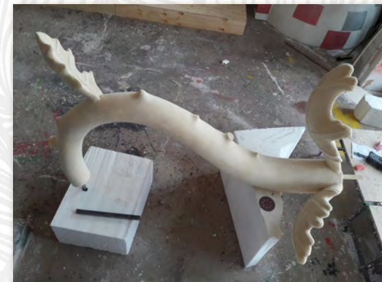
Polishing the surface of polystyrene
